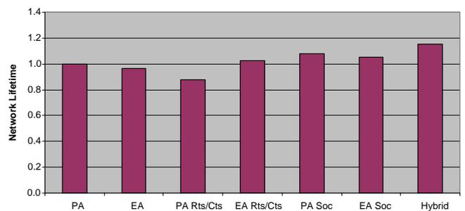
Fig. 8. Network life time for various position based routing implementations.
