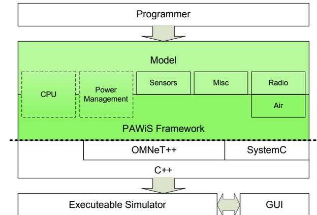
Fig. 1. Structure of the PAWiS simulation framework.
