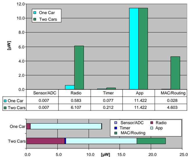
Fig. 7. Power consumption results of the TPMS simulation for one node.
