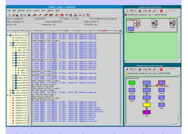
ule of the WSN node is implemented as C++ class derived from the PAWiS base classes. The modules are combined to the node with a configuration file. Another configuration file specifies the network layout. The simulator is built by compiling and linking the C++ files. It features a graphical user interface with step by step control of the module interaction. Alternatively a console application for high simulation speed can be built.
